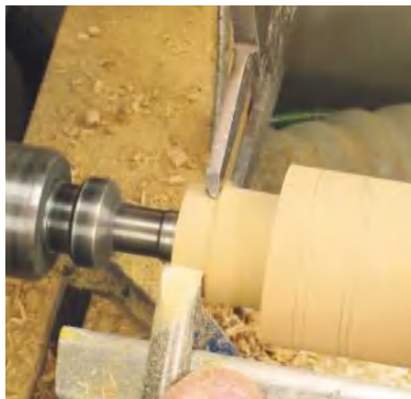
▲ Pic.17 Cut the spigot to fit into the base. Make sure this is accurate; a set of Vernier callipers will give you a more precise measurement over the bow leg variety
